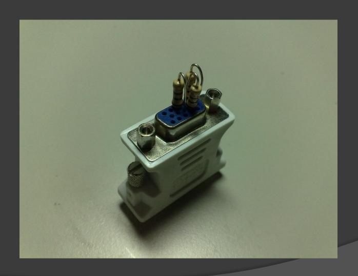
Use tape seal to fix the resistors for fear of coming off.
